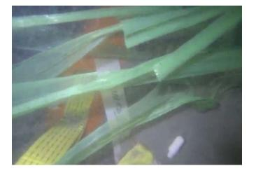
After 7 Days Buildup of sediment within the mattress area increases, reducing scouring
