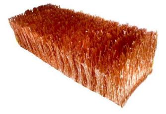
The Protech<sup>™</sup> Frond Mattress is a combined buoyant frond scour mat and flexible concrete mattress available in several standard variants, all featuring continuous and significantly overlapping parallel lines of buoyant fibrillated polypropylene fronds attached and aligned to the concrete blocks.
